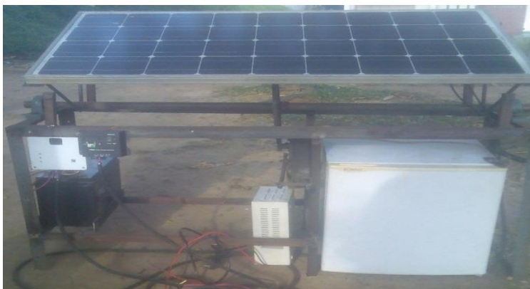
Figure 3. The Complete set-up of the Solar-Powered Refrigerator With Solar Tracker.
