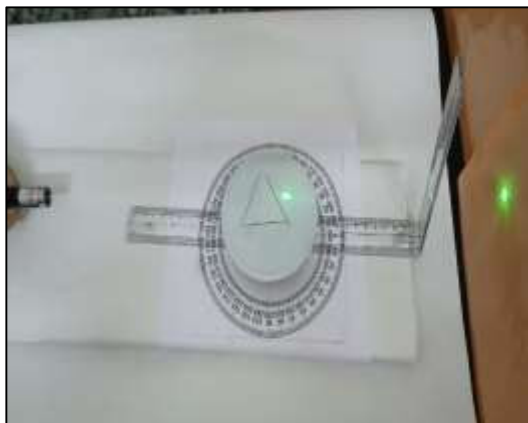
Figure 1. Undeviated Laser Beam in the absence of prism.
