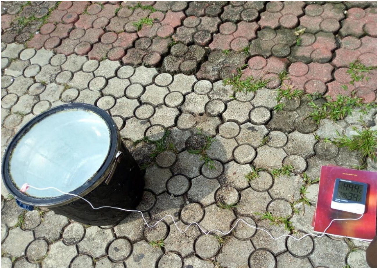
Figure 2. Testing of the solar bucket under the sun with a thermometer measuring the water in the solar bucket, the temperature of the environment, and the humidity.
