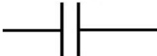
Figure 4. Basic symbol of a non-polarized capacitor.
