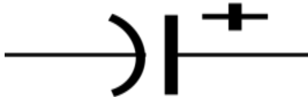
Figure 3. Basic symbol of a polarized capacitor.
