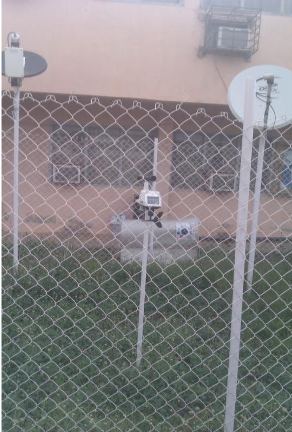
Figure 2(a). Diagram showing the outdoor unit of a MRR, Located at Physics Department, Federal University of Technology Akure.
