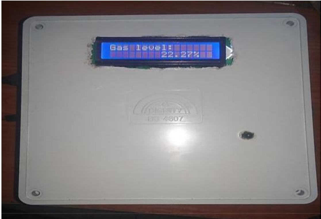
Figure 5. Gas Reading Display
