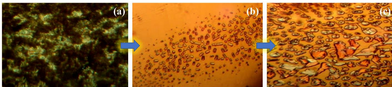
Figures 1. POM images of compound AB 9 : solid (a); Nematic phase (b); smectic phase (c).
