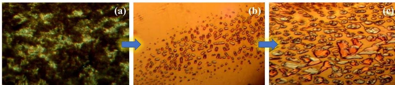
Figures 1. POM images of compound AB 9 : solid (a); Nematic phase (b); smectic phase (c).
